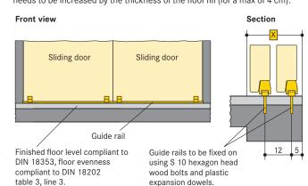
All dimensions shown are minimum. Constructional tolerances must be taken into consideration. All dimensions in cm.
